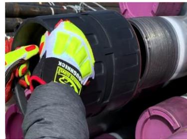
Note: The handlebar is considered to be “the integrated tool” for easy manual operation when required. By employing massive body weight and full force pull you might be able to rip the protector off. This force is not replicating normal handling of the tubulars.
